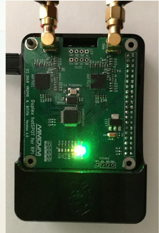
Duplex MMDVM on Raspberry Pi 3B DMR both slots
