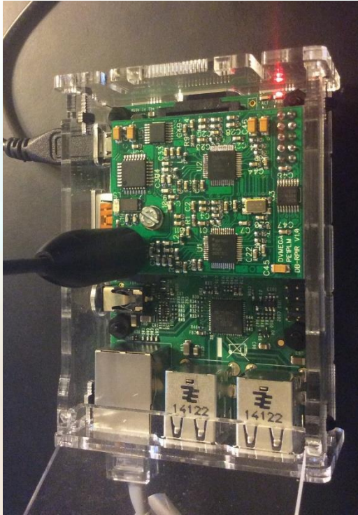
Dual Band DVMega on Raspberry Pi 2 D-STAR, DMR, YSF
